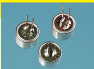
A Three electret microphones viewed from below. Upper right: from RadioShack. Upper left: from mouser.com . Bottom: from allelectronics.com . The ground terminal is on the right-hand side in each case.
