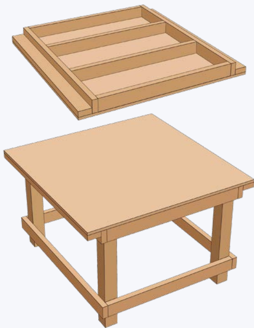
Fig. A: The tabletop is a 4'x4' sheet of \frac{3}{4} " plywood, braced and edged with 2x4s. The table legs are 4x4s. Fig. B: Two tables a couple of inches apart allow long cuts across big sheets of plywood or plastic, by running
