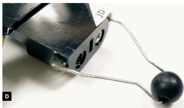
Fig. C: Switches and motor plate glued to the back of the battery holder. Fig. D: Bent paper clip threaded through a bead and glued to the rear end of the battery holder to make a rolling caster.
