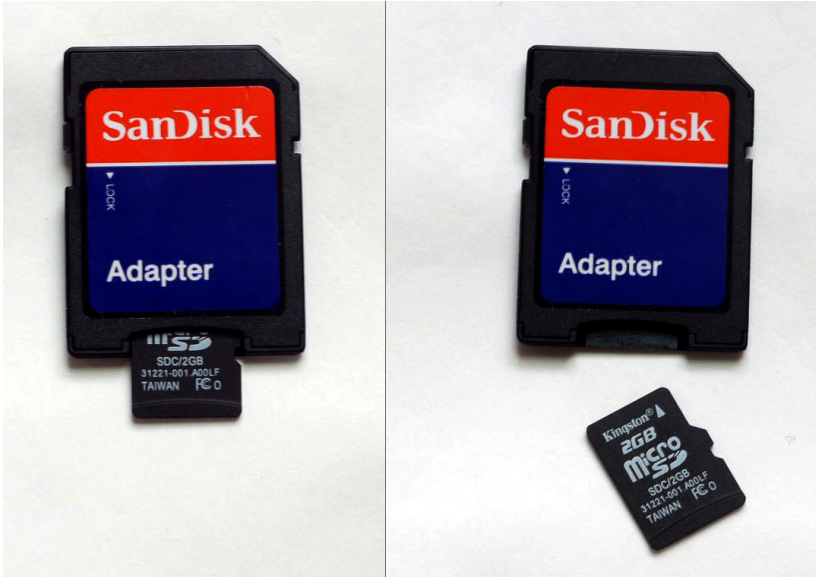
Figure 6-5. The MicroSD card can be moved between your Ethernet shield and an adapter sized for the typical SD card slot on a computer.
