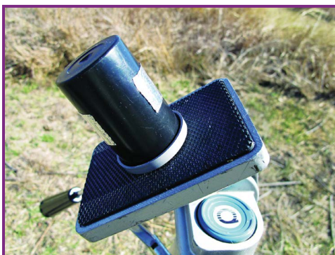
FIGURE 6-2. The film canister sunshine recorder can be mounted on a tripod by boring a \frac{1}{4} " hole in the lid and securing it to the tripod screw with a 3-40 nut.
