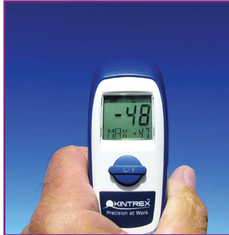
FIGURE 9-5. The inexpensive Kintrex IRT0421 infrared thermometer measuring the infrared radiation radiated down to the surface by the tiny amount of water vapor in the clear sky high over Hawaii’s Mauna Loa Observatory.
