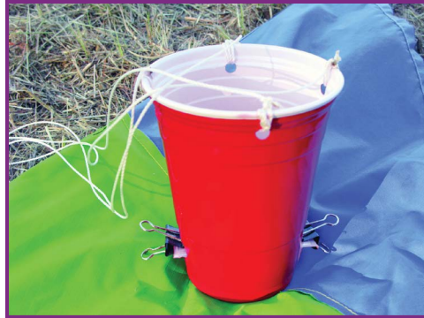
FIGURE 8-7. At the bottom of the air sampler, binder clips hold the microscope slide in place.
