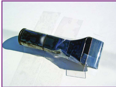
FIGURE 8-3. Air sampler made from a vacuum cleaner inlet fixture and a microscope slide.
