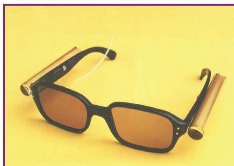
FIGURE 30-3. All the electronics were installed inside two 3/8"-diameter brass tubes mounted on the temples, the LED transmitter in one tube and the receiver in the other. A tiny hearing aid earphone in the receiver tube was coupled to the user's ear through a short length of plastic tubing.
