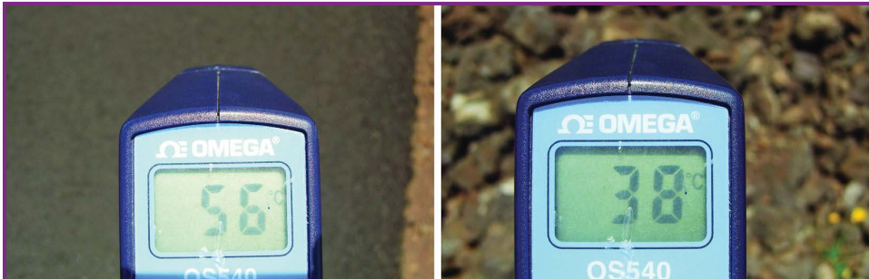
FIGURE 7-1. Paved sections of Hawaii’s Mauna Loa Observatory road (left) are much warmer than nearby lava rock (right), presumably because of the lava’s porosity.
