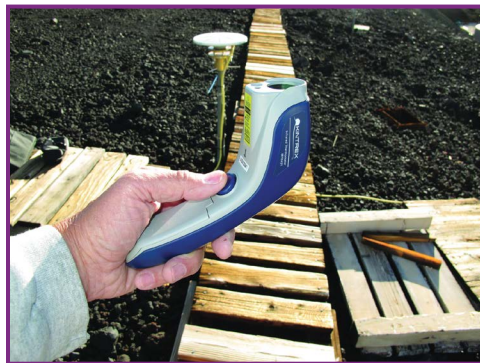
FIGURE 9-6. The author recently calibrated 7 infrared thermometers against the NOAA GPS water vapor receiver (white disk on pole) at Mauna Loa Observatory.
