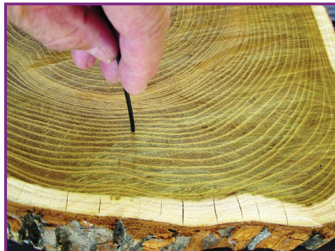
FIGURE 25-8. Using the PAC light probe to scan the rings of a bois d'arc tree felled by a flood.
