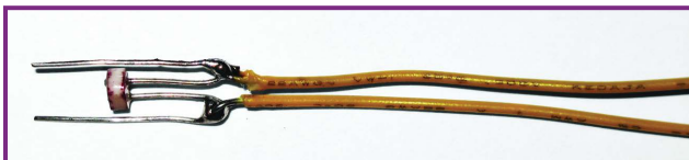
FIGURE 25-2. Breadboard-style connection leads are soldered to the photoresistor leads.
