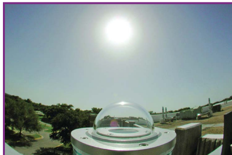
FIGURE 14-4. UV-B data from this U.S. Department of Agriculture radiometer at Texas Lutheran University at Seguin, Texas, are online.
