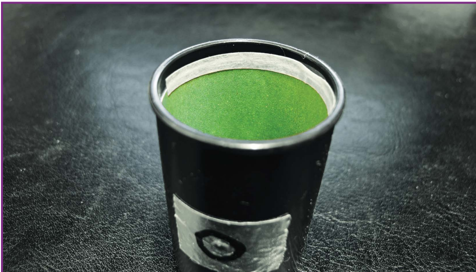
FIGURE 6-1. Pinhole sunshine recorder made from a plastic 35mm film canister. A thin strip of masking tape holds the blueprint paper in place.
