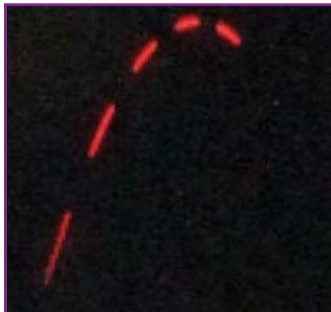
FIGURE 23-6. Time exposure shows the apogee of a flight neatly outlined by a red LED flasher.
