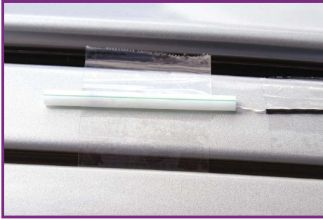
FIGURE 3-6. Insert the sensor into the tube's forward opening, tape its cable to the door frame, and run the cable through the window.
