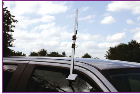
FIGURE 3-7. Remove the cap and the flag. Extend the sensor just beyond the upper end of the flagpole and secure it by wrapping a few inches of insulated, solid wire around the sensor leads and the groove at the top of the flag mount. Use tape or binder clips to secure the cable to the flagpole.
