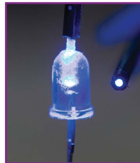
FIGURE 24-6. Bare fiber inside a blue LED.
