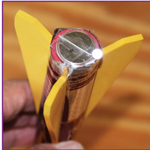
FIGURE 23-4. LED throwie taped to a Sky Rocket.
