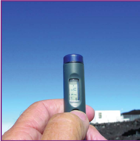
FIGURE 9-4. The inexpensive Kintrex IRT0401 infrared thermometer measuring the infrared radiation radiated down to the surface by the tiny amount of water vapor in the clear sky high over Hawaii’s Mauna Loa Observatory. Sometimes the sky is so dry that there is too little radiation to be measured by these IR thermometers.
