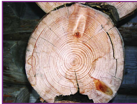
FIGURE 1-5. This Norway spruce log was used to build a cabin in Switzerland. Experienced dendrochronologists can compare these rings with those of logs with known dates to determine when this log was cut.
