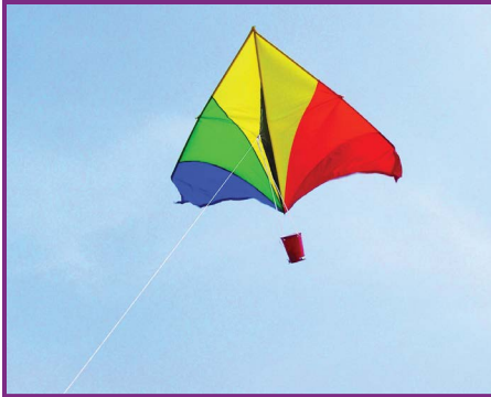
FIGURE 8-6. A DIY passive air sampler flies from a delta kite at Padre Island, Texas, to capture spores in smoke from agricultural fires in Yucatan.
