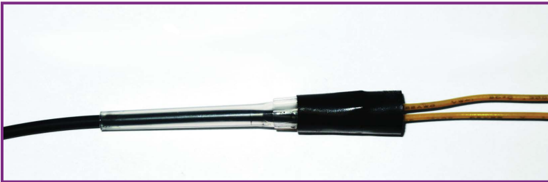
FIGURE 25-4. Assembled PAC light probe. The backside of the probe should be blocked from external light.
