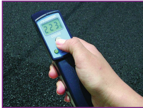
FIGURE 7-3. Sarah Mims measured a newly paved asphalt road at nearly 225°F during a heat island study.
