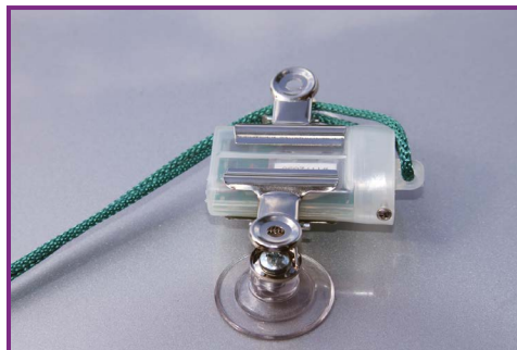
FIGURE 3-5. Mount an Onset Pendant logger on a car roof with a pair of Adams suction cup clamps and a safety line.
