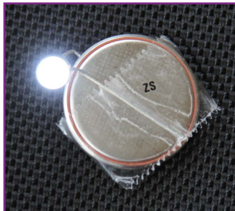
FIGURE 23-3. The simplest LED device, an LED throwie, made by taping an LED to a coin cell battery.
