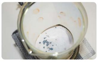
FIGURE 22-4: Fingerprints developed by iodine fuming
