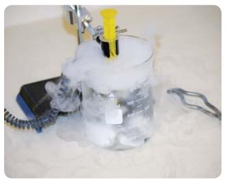
FIGURE 14-3: Measuring gas volume in a bath of alcohol and dry ice
