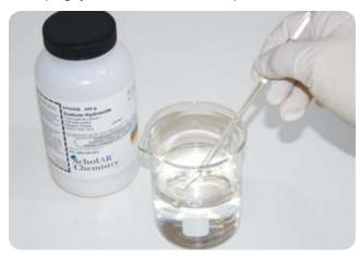
flasks are made of Pyrex or similar glass, there's no reason to risk your volumetric flask. For an accurate measurement, you need to allow the solution to cool to room temperature anyway, so you might as well make up the solution in a separate container, as shown in Figure 5-6, and do a quantitative transfer to the volumetric flask once the solution has cooled.
