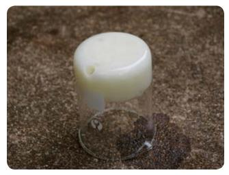
8. If you are not already outdoors, take the beaker to a safe outdoor location with a nonflammable surface such as dirt, gravel, or concrete. (Remember that asphalt, made from tar, is flammable.) Invert the beaker, and wait a few moments to see whether the gelled sol separates from
