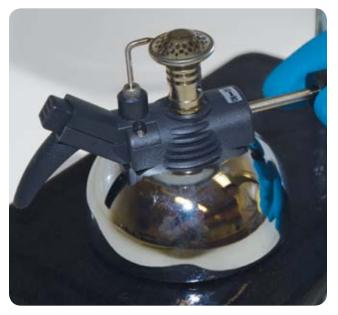
These burners have internal fuel storage, and are filled from inexpensive disposable butane canisters sold by drugstores and tobacconists. Most run for an hour or more at their highest setting on a full tank of fuel. Because they are not tethered to a natural gas tap, you can move these burners around the lab as needed. Flame spreaders and other accessories are often available for such burners, either included with the burner or as options.
