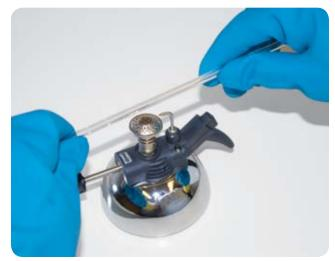
A good bend is one in which the tubing assumes the desired angle smoothly with no internal crimping or constriction. If you haven't heated the tubing sufficiently, the bend will be uneven. If you've overheated the tubing, the bend may be too sharp and there may be a constriction or blockage at the most extreme part of the bend.
