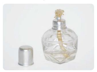
when you are trying to reduce a metal ore with carbon, the higher temperature of the gas flame may be necessary to initiate and sustain the reaction. (If you have no gas burner, you can increase the temperature of an alcohol lamp flame significantly by using a blowpipe or a piece of glass tubing to blow air into the flame.)
