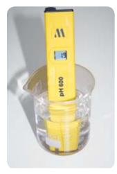
Using a pH meter to determine the pH of a solution
