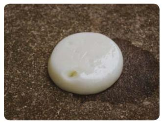
the beaker. If not, tap the beaker gently to release the gelled sol. When the gelled sol separates, note that it retains its form, as shown in Figure 18-5. There should be little or no liquid gasoline remaining. (The stain visible to the right of the gelled sol in Figure 18-5 is a small amount, probably less than 1 mL, of liquid gasoline that was not incorporated in the sol.)
